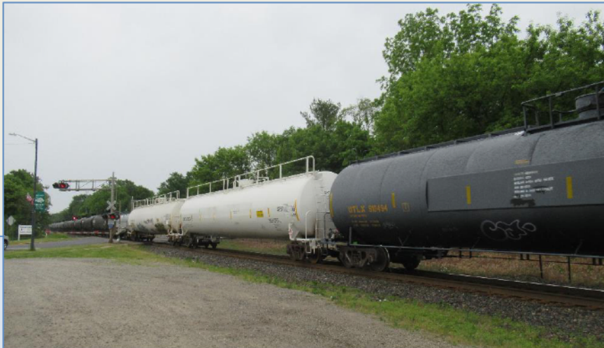
WB DOT 112 tank cars with UN 1975 at Marcellus, MI 6-8-2022 photo by Rich Mahaney
