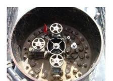
Pressure Tank Car Valve Examples – common for LP gas and anhydrous ammonia. Liquid valves, vapor valve, pressure relief device, gauging devices, sample line, thermometer well
