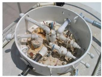
Example of piping for a pressure car under the cover—long pipes are for liquids (in and out), magnetic gauging device (silver ball), short pipe at top is the vapor line, two smaller pipes are the sample line and the thermometer well.
