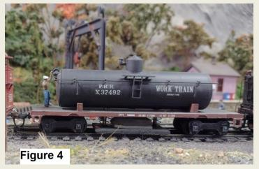
I built a track-cleaning car that is just a freight car with a piece of Masonite (rough side down) that rests on the rail under the car. This lives on a MOW train that I run before every OPS session. Some folks advocate having 3 or 4 cars equipped with this rig wandering around the layout. This is an old technique that's been around since the 1950s, I think.
