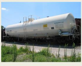
DOT-114 Tank Car (with spray on insulation and no jacket)
