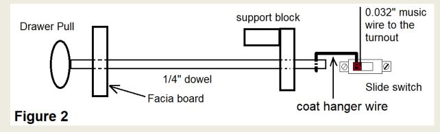
In this case the switch is mounted horizontally under the layout. 2 holes are drilled in the switch one for the 0.032'' wire going up through a 1/4'' hole to pierce the throw bar and a larger hole to connect the switch to a length of 1/4'' dowel. Then to operate the turnout one just pulls or pushes the knob which moves the switch and the turnout. **(Figure 2)**
