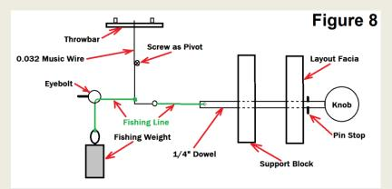
I've even seen auto choke cables used to control turnouts in the larger scales.
