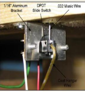
the switch handle that extended through a hole to pierce the throw bar from below. This is the same way that a tortoise machine operates a turnout. **(Figure 2)**
