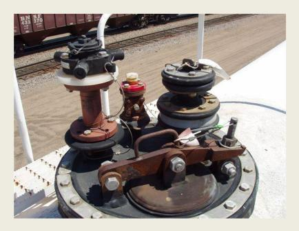
Photo #24 – shows an example of "shelf couplers" that are placed on all tank cars at this time.
