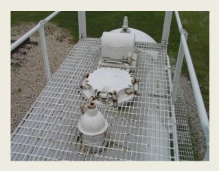
Photo #22 – shows a "Top Operated Bottom Outlet Valve" on a low-pressure tank car. It is also known as a "TOBOV" valve. It works to open a valve or drain on the bottom on a the bottom of a tank car.
