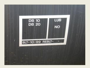
Photo # 10 shows an example of a "built date" on a tank car. This is when this car was constructed, which is important relating to the type of steel was used.
