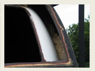
Photos #12 and #13 – show the differences between a "jacketed" and "non jacketed" tank car. You can see in one case how the bolster is welled to the tank. In the other photo that is covered up by the "Jacket".
