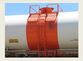
**Photo # 6 Cryogenic Tank Cars**
