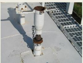
Tank Car Valves - TOBOV Top Operated Bottom Outlet Valve
