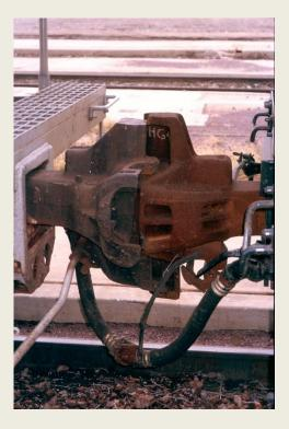
Photo #25 – Shows the "pin" that sticks into the bottom of a rail car (in this case a tank car) that keeps the wheel set "attached" to the rail cars. The weight of the cars keeps the wheel set attached to the rail car.
