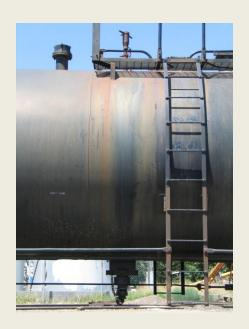
Photo #23 – shows the equipment used for loading and unloading a tank car transporting corrosive liquids. The safety relief equipment is also shown.
